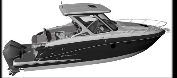
LOA: 31' 2" OVERALL LENGTH WITH ENGINES: 32' 11" **BEAM: 116"** MAX DRY WEIGHT: 13,000 LBS DEADRISE: 19° FUEL: 135 GALLONS **MAX HP: 800**
