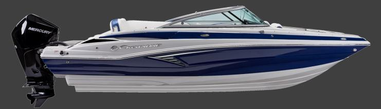
OVERALL LENGTH W/ENGINES: 23' 9" LOA: 21' 4" BEAM: 102" MAX DRY WEIGHT: 4060 LBS DEADRISE: 19° FUEL: 45 GAL MAX HP: 250
