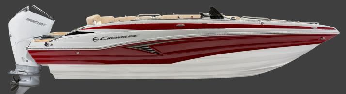
**OVERALL LENGTH W/ENGINES: 24' 5"** LOA: 21' 10" **BEAM: 102"** MAX DRY WEIGHT: 4125 LBS **DEADRISE: 19°** FUEL: 55 GAL **MAX HP: 250**
