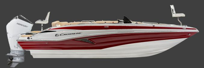
OVERALL LENGTH E/ENGINES: 24' 5" LOA: 21' 10" BEAM: 102" MAX DRY WEIGHT: 4125 LBS DEADRISE: 19° FUEL: 55 GAL MAX HP: 250
