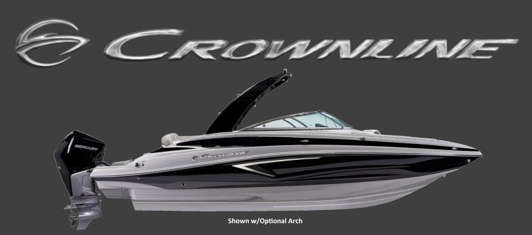
OVERALL LENGTH W/ENGINES: 27' 7" LOA: 25' 3" BEAM: 102" MAX DRY WEIGHT: 5275 LBS DEADRISE: 19° FUEL: 55 GAL MAX HP: 350
