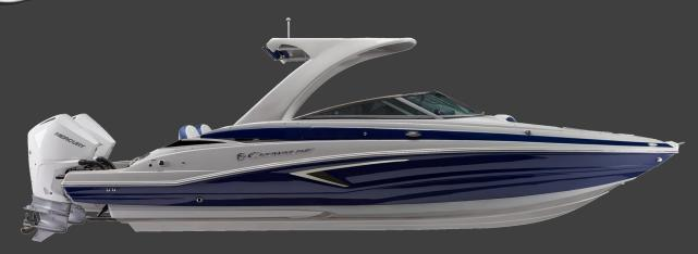
OVERALL LENGTH W/ENGINES: 31' 8" LOA W/OUT ENGINES: 29' 3" BEAM: 110"
