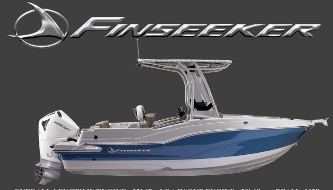
OVERALL LENGTH W/ENGINE: 22' 6" LOA W/OUT ENGINE: 20' 6" BEAM: 102" MAX DRY WEIGHT: 4295 LBS DEADRISE: 19° FUEL: 75 GAL MAX HP: 225
