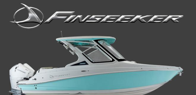
OVERALL LENGTH W/ENGINES: 28' 11"LOA W/OUT ENGINES: 26' 10"BEAM: 112"MAX DRY WEIGHT: 8900 LBSDEADRISE: 22°FUEL: 170 GALBAITWELL: 26 GALMAX HP: 600
