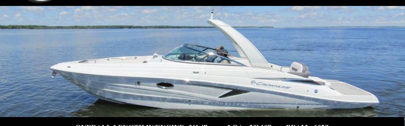
OVERALL LENGTH W/ENGINE: 31' 4" LOA: 28' 10" BEAM: 102" MAX DRY WEIGHT: 6025 LBS DEADRISE: 23° FUEL: 78 GAL MAX HP: 425
